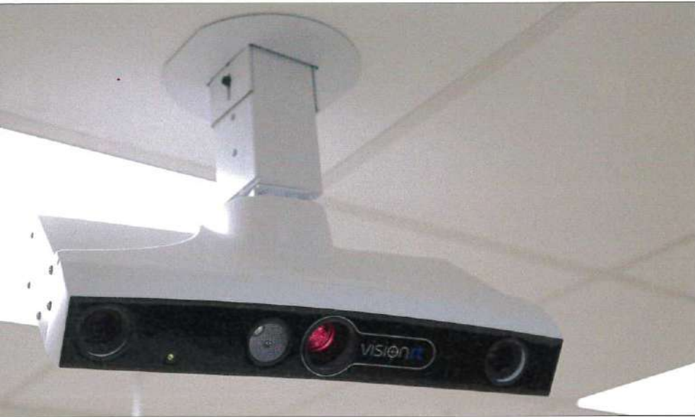
Ceiling-mounted modules contain a projector and stereoscopic camera. These need to be precisely aligned
