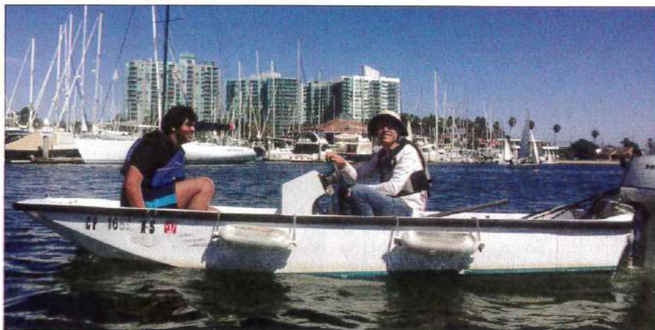
The call of the sea University of California, Los Angeles graduate students Shashank Gowda and Muchen Xu are testing superhydrophobic surfaces attached to the bottom of a motorboat in Marina del Rey, California.
